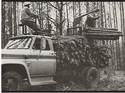
Figura 7. Bobtail truck provisto de un big stick loader .
